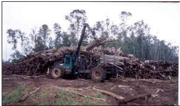
Figure 6.5 Short distance wood transportation and wood loading using forwarder in one HTI in Sumatera
