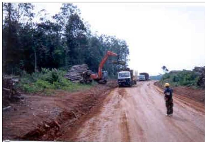
Figure 6.6 Wood loading and unloading using grapple loader
