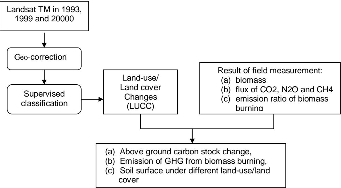
Fig. 2. Flowchart of Analysis Step
